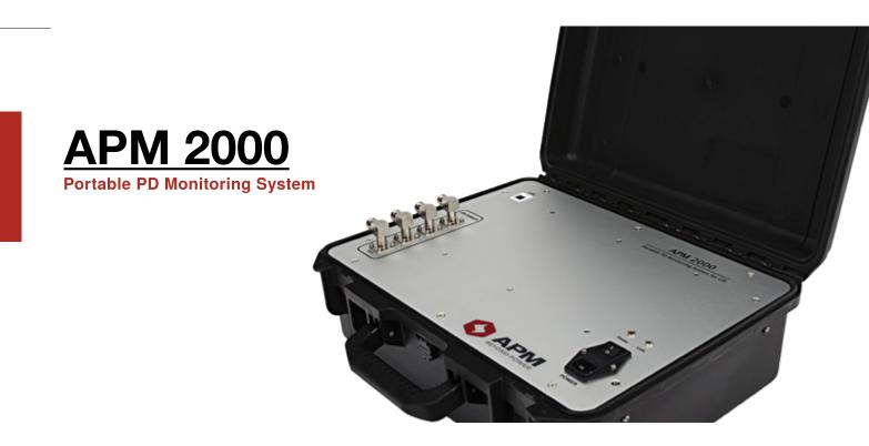
APM 2000 detects and alerts various defects inside EHV/MV equipment by analyzing UHF signals generated by partial discharge. It monitors, records and analyzes PD signal continuously and alerts the condition of EHV/MV equipment with light-weight and small-sized equipment.
