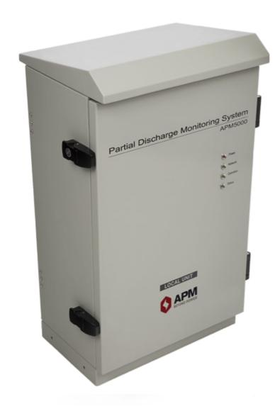
APM5000 detects and alerts various defects inside GIS by analyzing UHF signals generated by partial discharge that can cause progressive deterioration of insulating materials, ultimately leading to electrical breakdown.
