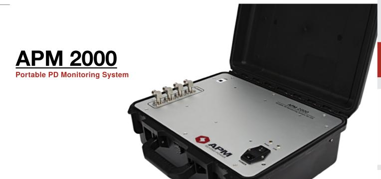
APM 2000 detects and alerts various defects inside GIS by analyzing UHF signals generated by partial discharge. It monitors, records and analyzes PD signal continuously and alerts the condition of GIS with light-weight and small-sized equipment.
